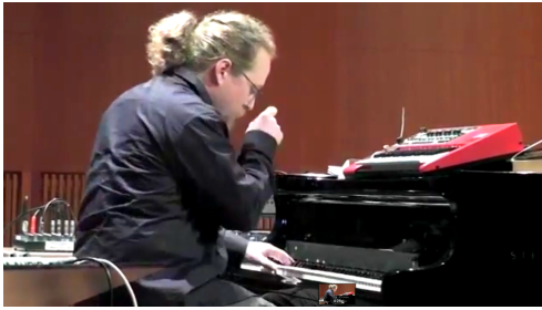
Figure 1: A picture from the premiere of the Foldings system in 2011. The red machine on top of the grand piano is the Nord G2 signal processing engine. It does both mapping and sound processing, but is not interacted with directly during the performance. Later performances have used a smaller version without interface, hidden behind the performer. The Moog Piano Bar MIDI sensor can be seen on top of the keys, against the keyboard lid.
