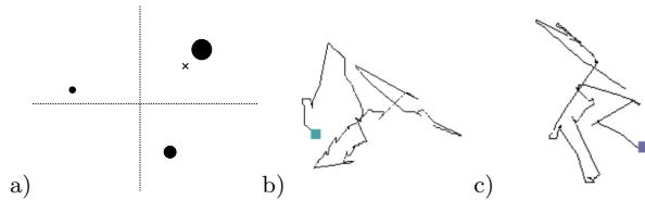
Figure 2: a) An illustration of the gravity model. When several notes, each corresponding to a point in synthesis parameter space, are played with different velocities, they attain different gravities. A louder note will have a larger attraction effect on the resulting point (the small cross). This illustration is greatly simplified. In the real system, the gravities vary over time, following attack, decay and release settings, and the process takes place in an 8 or 16-dimensional parameter space. Fig. b) and c) show 2D projections of real trajectories (each of 10 sec duration), taken from video example 4, where also the simultaneous control of 8 parameters can be seen and heard.
