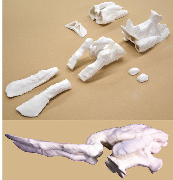
Figure 4. Nasal passages. Divided into smaller pieces for printing (above), assembled and epoxy infiltrated (below)
