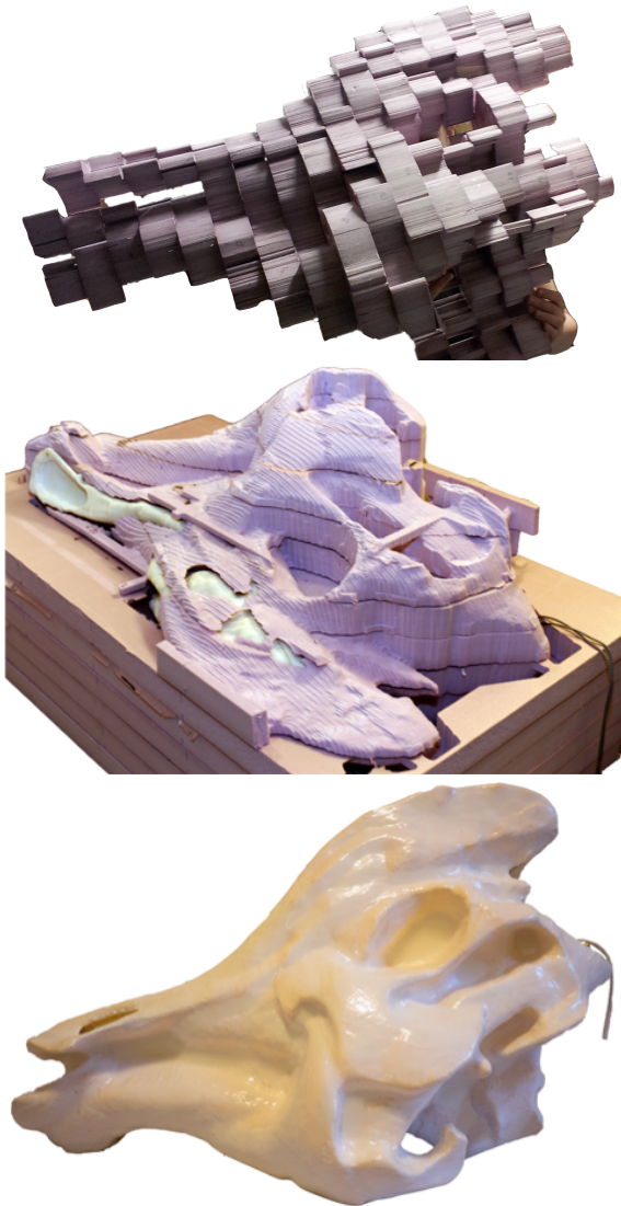
Figure 5. A progression of outer skull prototypes. Top: Prototype I assembled from 5cm thick foam sections. Middle: Prototype II assembled from 5cm thick section of CNC machine foam. Bottom: Prototype III from a block of EPS foam, coated in epoxy, forming the resonant body.
