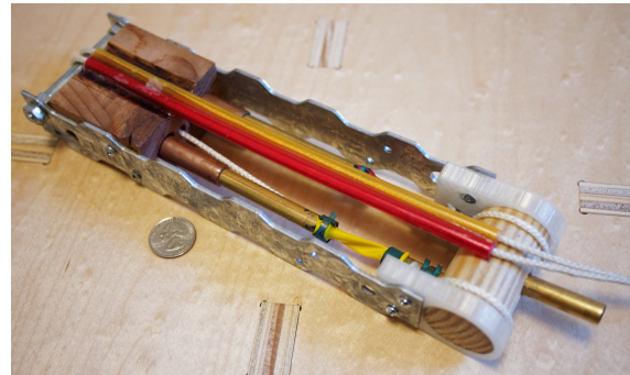
Figure 3. The final version of the larynx, showing one of the two balloons (yellow), with a quarter for scale. The mouthpiece is on the right. The strings pull on the balloons.
