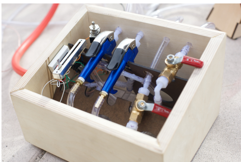
Figure 5: The exposed interior of Controller 2, housing two blow guns and two ball valves.
