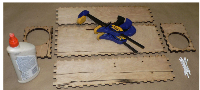
Figure 2: Preparations for gluing together pieces of laser-cut plywood to make an enclosure.
