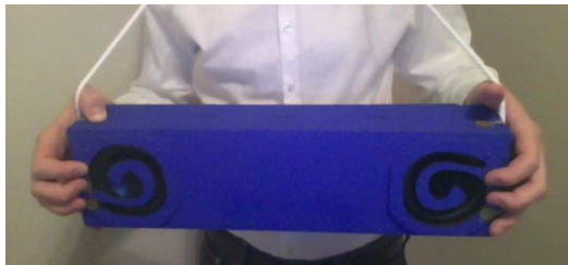
Figure 6: “The SuperSonicSoaker soaks you with sound.” It is a derivative of the LapBox revision 4 that is designed to be held by a strap going around the neck.
