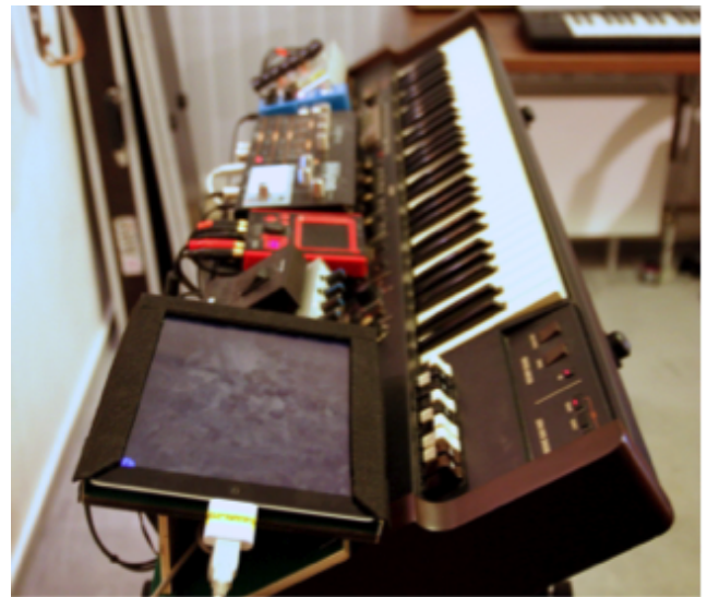
Figure 6: The evaluation setup - a standard, commercially available synthesizer (black device in the center) that is connected to the keys of an organ and a framed tablet (front) that provides the touch interface presented in this work. The other boxes in this picture were not used during the evaluation.
