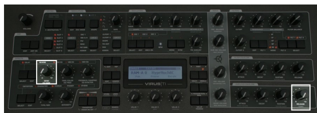
Figure 2: On the Access Virus TI2, the reverb knob is on the left, while the amplifier release time knob is on the bottom right.
