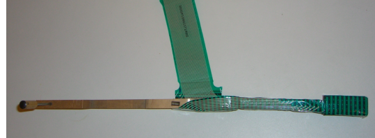
Figure 11: Prototype of a flexible PCB based FSR, 4 x 28 matrix sensor attached to the top of a piano key. The sensitivity is around 40gr and the sampling frequency is 100Hz.
