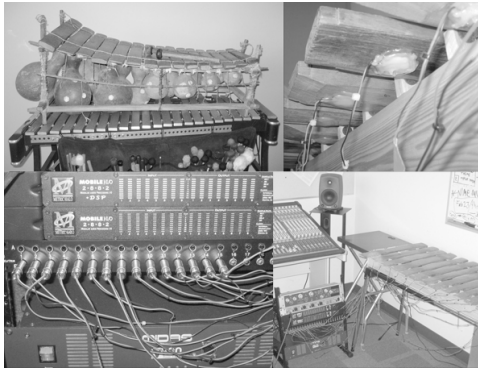
Figure 1: Top left: Gyl on top of vibraphone for showing scale, Top right: piezo sensors under bars, Bottom Left: 2882 input, Bottom Right: overview
