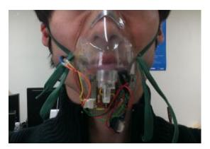
Figure 1. Respiration sensor device
