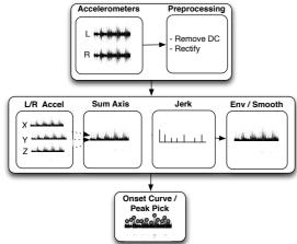
Figure 3 - Overview of Onset Detection Algorithm
