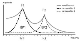
Figure 5. Using two band-pass filters to shape source signal into human formant like spectral shape.
