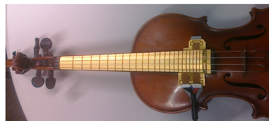
Figure 2: Switch matrix sensor for left hand finger position sensing. A flexible PCB is mounted on the violin finger board. The contact areas are coated with gold.
