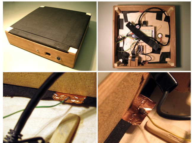
Figure 3: Fab : conductive fabric drawing board
