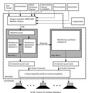
Figure 1. The hardware and software infrastructure for *Windtraces*.
