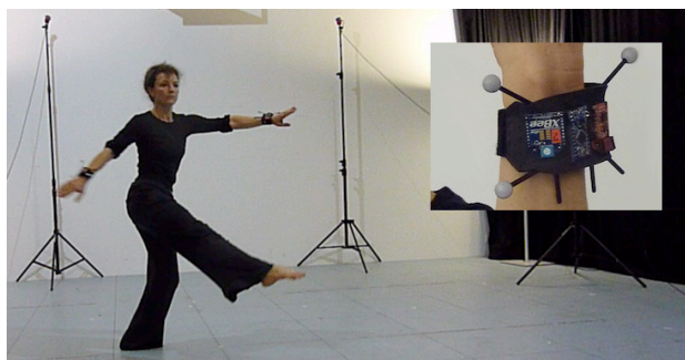
Figure 1. The dancer in our lab wearing accelerator bracelets and motion-capture markers on her wrists. The insert shows one of the bracelets in combination with a rigid-body marker used for motion capture.
