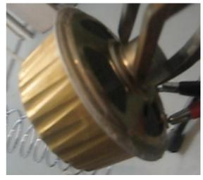
Figure 4. Foil cup prepared speaker
