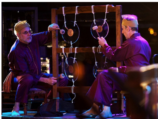
Figure 4: Gamelan ElektriKA gongs being performed by Mark Stewart and Jacques Weissgerber. Rear mounted piezos discs are used to detect the strike while centered gold discs provide damping through capacitive sensing. Photo by Kevin Yatarola
