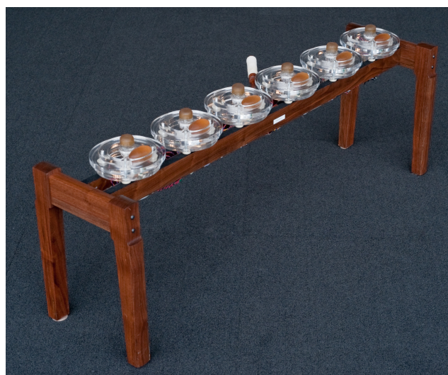
Figure 3: One half of the reong holding six pots. The center is a free-standing rod with piezo films and FSRs placed underneath used to implement byongs . The small pads on the right are the chucks .
