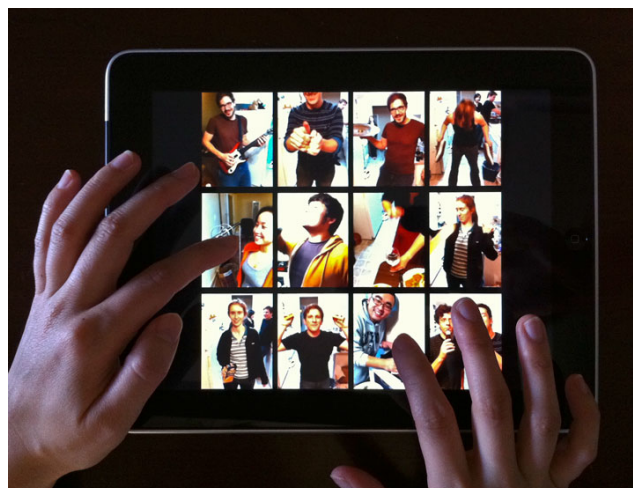
Figure 1: MadPad in action on the Apple iPad. The performer taps on the video clips to play the associated audio and video.
