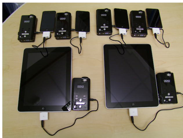
Figure 4: An ensemble setup of mobile projectors and their driving mobile devices.
