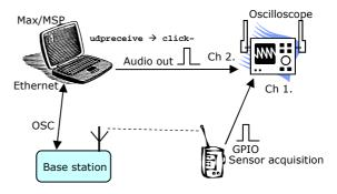
Figure 3. Latency measurement technique
