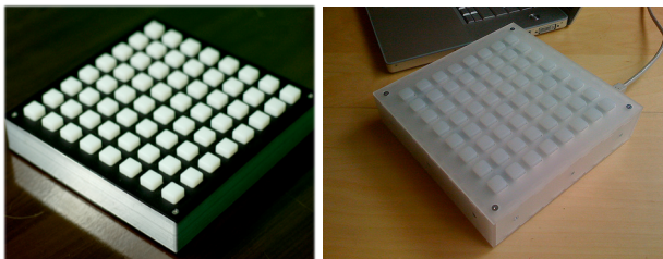
Figure 2: Arduinomes using two separate silicon buttons
