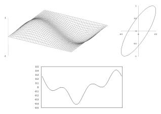
Figure 4. Wave terrain synthesis, (i) terrain, (ii) trajectory and (iii) time-varying output signal.
