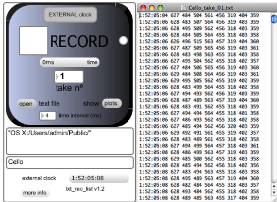
Figure 2. Sensor data recording object for Max/MSP (left) and example of recorded txt file with TC (right)
