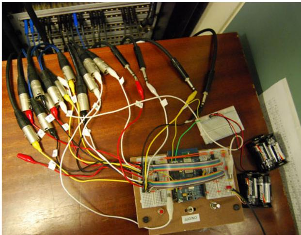
Figure 5. Arduino connections to the Sonic Lab's patch panel
