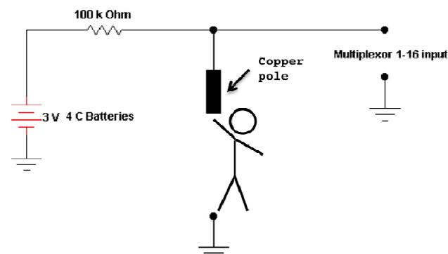
Figure 4. Electrical circuit used to measure people's impedance
