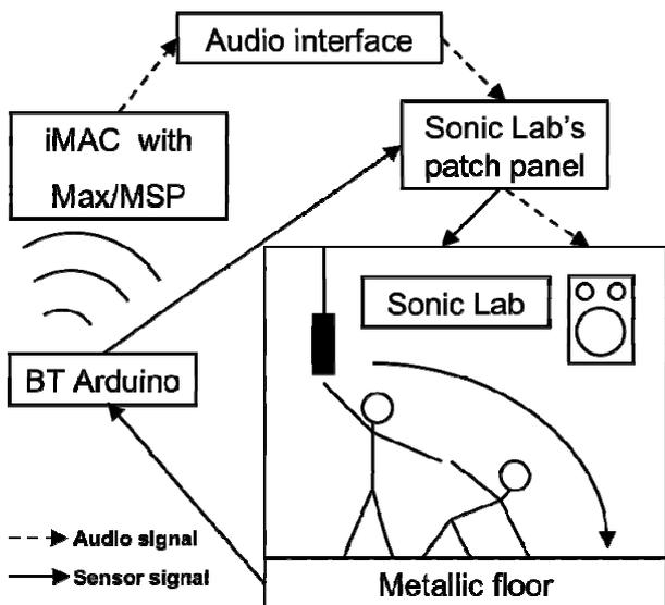
Figure 6. Signal flow diagram for Ground Me!
