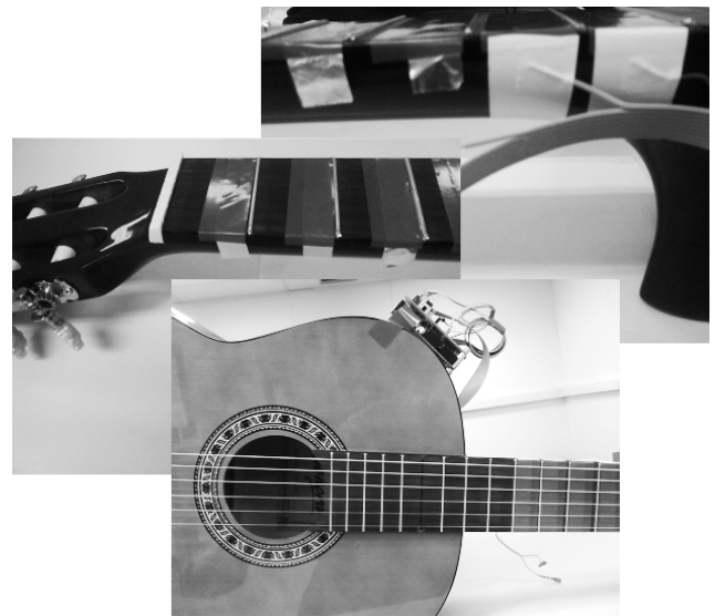
Figure 1: Non intrusive capacitive sensors mounted on the first 10 frets of a nylon guitar. The Arduino is attached to the guitar's body to reduce background noise and increase stability.
