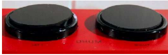
Figure 6: The hitting exciter is implemented with two drum pads. Inside each drum pad there is a pressure sensor, which picks up the force applied by the user.
