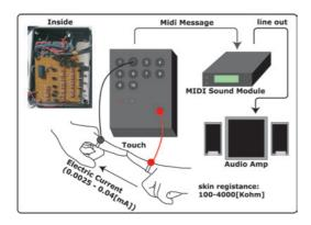
Figure 3: Overview of Freqtric Drums system.
