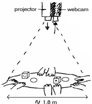
Figure 6. The *reacTable*\* simplified scheme
