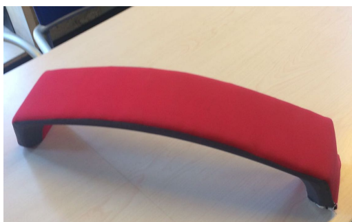
Figure 3: Third prototype, Arcontinuo 1512, 3D printed and covered by polyester.
