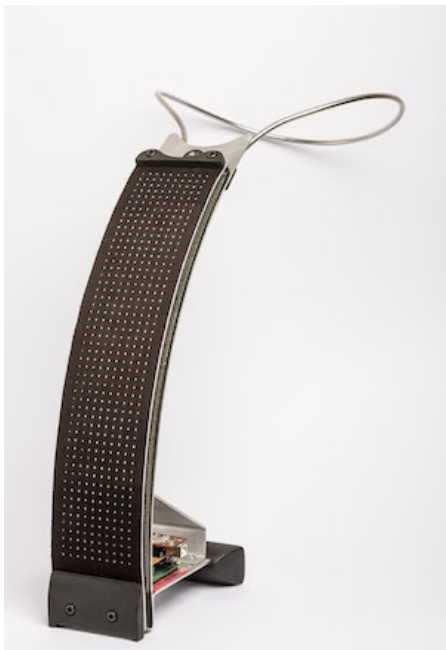
Figure 2: Second prototype, Arcontinuo 520, made of aluminum, silicone and lycra.
