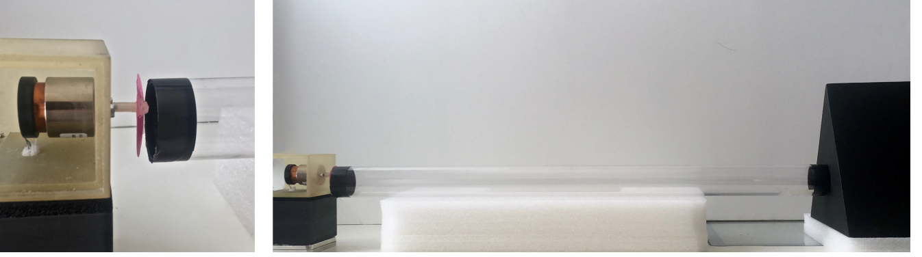
Figure 2: Aerophone Prototype Instrument (right), voice coil motor attached to an articulated damper (left).
