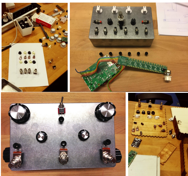
Figure 2: Photos taken during the workshops, while participants design their layout for the front panel, either on paper (top left) or on the enclosure, by arranging the caps of knobs.
