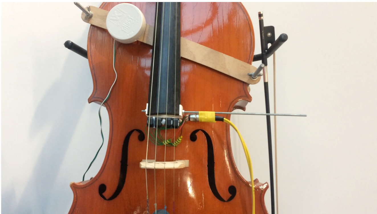
Figure 2: The four pickups are held in a 3D printed mount which attaches to the end of the finger board. A transducer is braced on the upper front body
