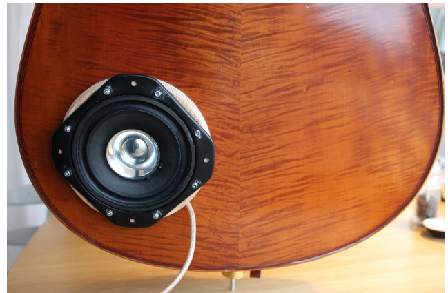
Figure 4: A 50W speaker is built into the back of the cello body, mounted on a spruce collar to maximise vibrational conductance.
