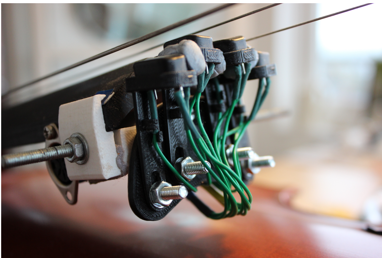
Figure 3: Close up of the pickup mount which allows vertical and rotational adjustments. The blue tack in this prototype prevents oscillations in the plastic arms of the individual mounts which can themselves become the dominating frequencies if undamped.
