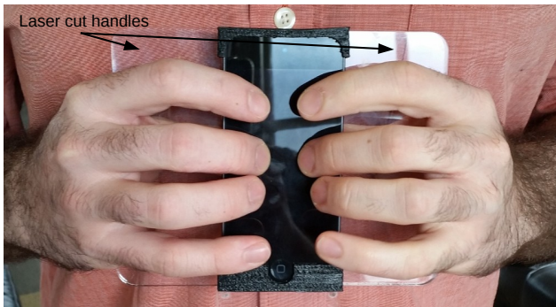
Figure 9: Smart-phone augmented to be held as a wind instrument.
