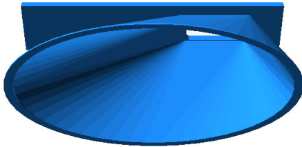
Figure 1: CAD model of a generic passive amplifier for the built-in speakers of a mobile device.
