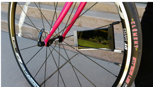
Figure 13: Mobile device mounted on a bike wheel (instrument by Patricia Robinson).
