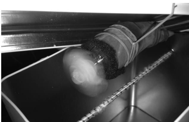
Figure 5: The motor striking the string of the instrument.
