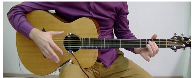
Figure 5. Performing with the active acoustic guitar; the sound drivers are not visible and all sounds emanate from the guitar itself. Leap Motion sensor is used for hand gesture tracking mapped to sound processing.
