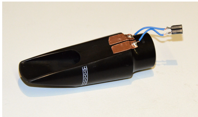
Figure 3: Alto-Saxophone mouthpiece by Otto Link with Copper Foil layer on the mouthpiece table, to connect the Fiber sensor reeds.
