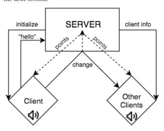
Figure 2: Monad v0.2 network structure for individual clients.
