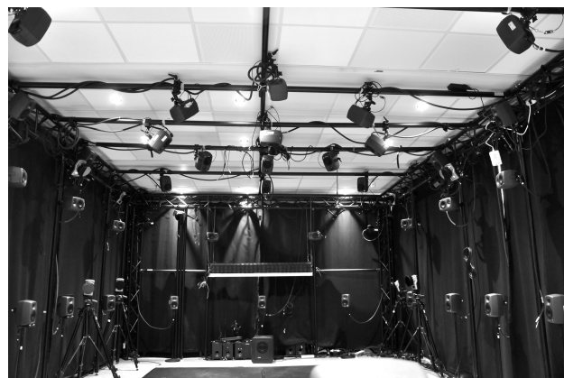
Figure 2: The 3-D Ambisonics array at the Department of Musicology, University of Oslo
