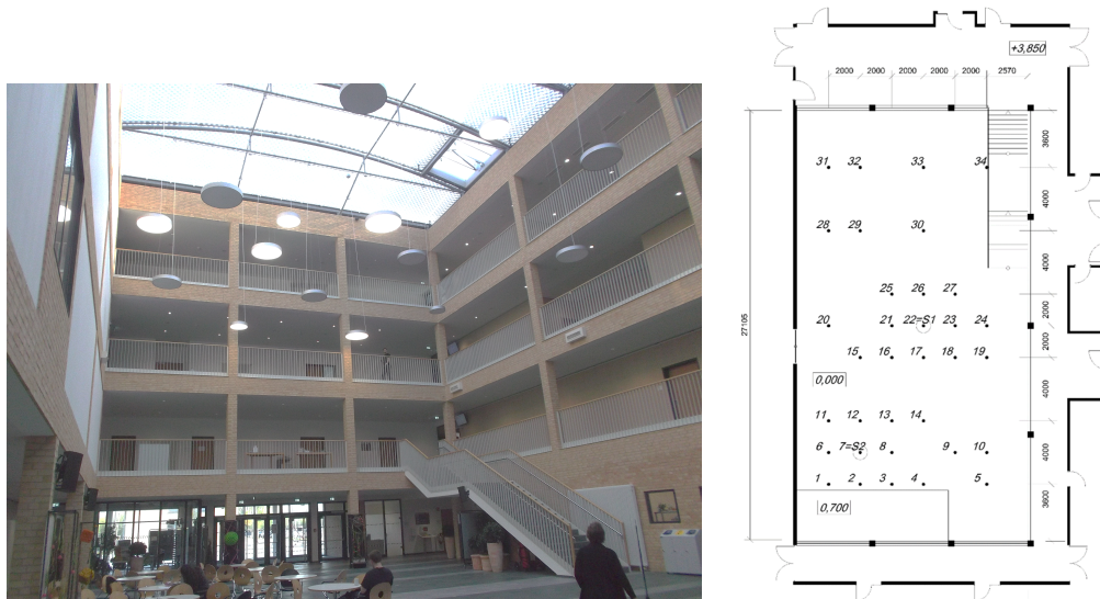
Figure 1. Positions of the sound source and microphones during the in-situ measurements (left), View of the atrium interior with Texlon ® ETFE roofing system.
