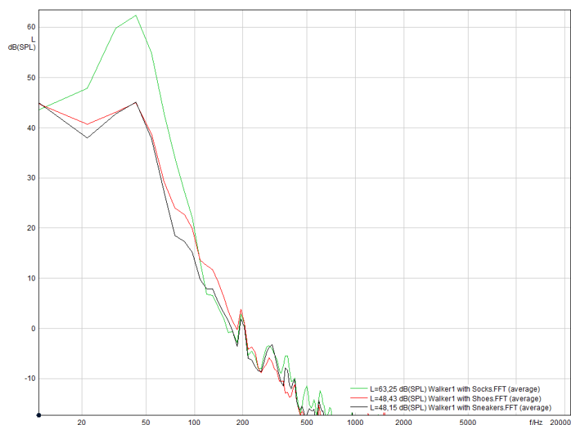
Figure 6. The spectra of footsteps sounds produced by the heavy walker on the massive floor, wearing only socks (green curve), casual shoes (red), and sneakers (black), walking at 75 steps/minute
