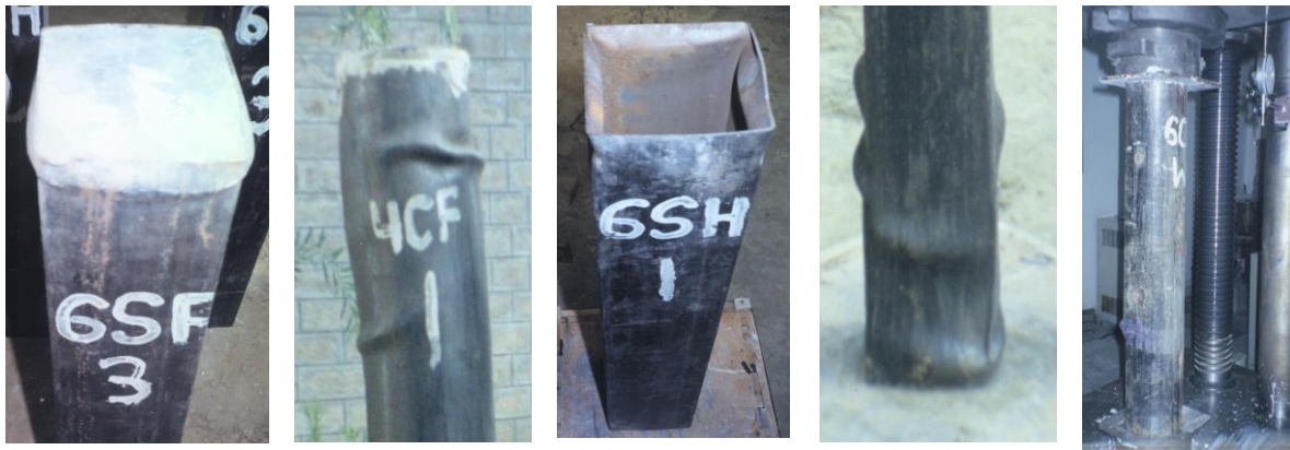
Figure-2. Photographs showing failure modes And test setup of columns
