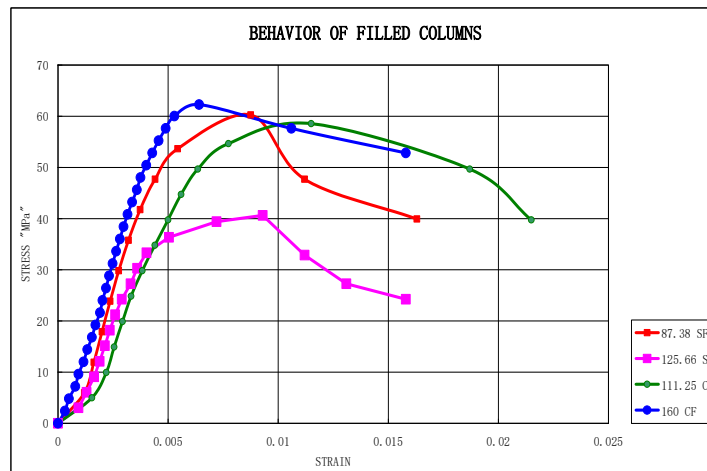
Figure 4. Stress – strain curve of filled columns
