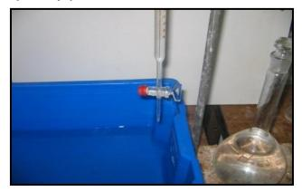
Fig 2. Correction of the sulfate solution by adding small quantities of 0.1N H<sub>2</sub>SO<sub>4</sub>, up to a pH equal to 6-8.
