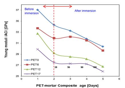
Fig 3. Evolution of Young modulus with volumetric PET rate and composite mortar ages via ACI-318 code
