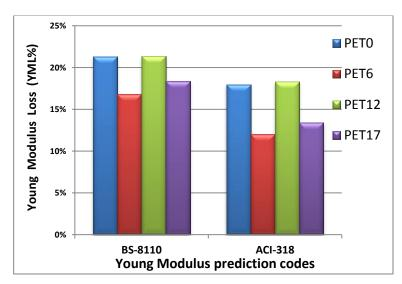
Fig 5. Young modulus loss (YML%) with volumetric PET rate and prediction codes (BS-8110 & ACI-318) before and after MgSO<sub>4</sub> immersion
