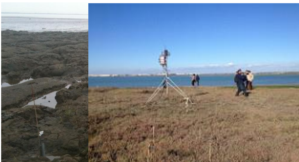
Figure 18 (left) Bed-mounted pressure sensor (see arrow) with buried cable connection to (right) telemetered data logging system at the Year 2 site in Cadiz Bay, ES.
