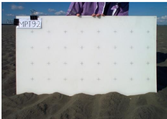
Figure 15 Example of a photograph with a properly clean (and thus white) roughness board.
