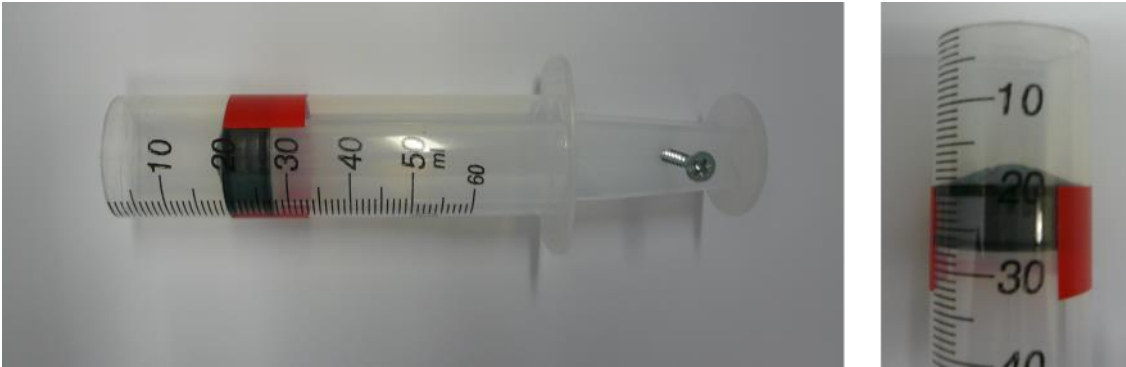
Figure 16 Sediment sampling with the big syringe, sides of the plunger should be level with top of the red tape to sample the right volume, as shown here.
