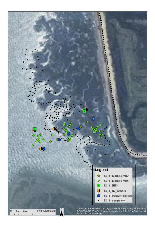
Figure 5: Locations of topographic surveys, monitoring equipment and sampling quadrats deployed at ES Y1 site
