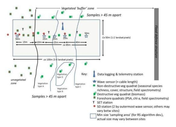
Figure 3: Schematic illustration of field sample layout used within the FAST project. Individual site locations vary from this and geo-referenced information of each sensor location is provided to accompany the wave measurement data uploaded on the FAST data repository.
