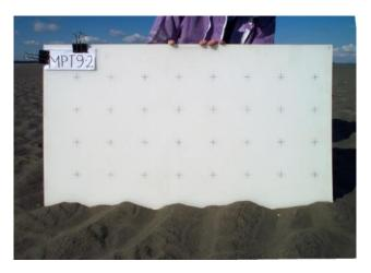
Figure 15: Example of a photograph with a properly clean (and thus white) roughness board.
