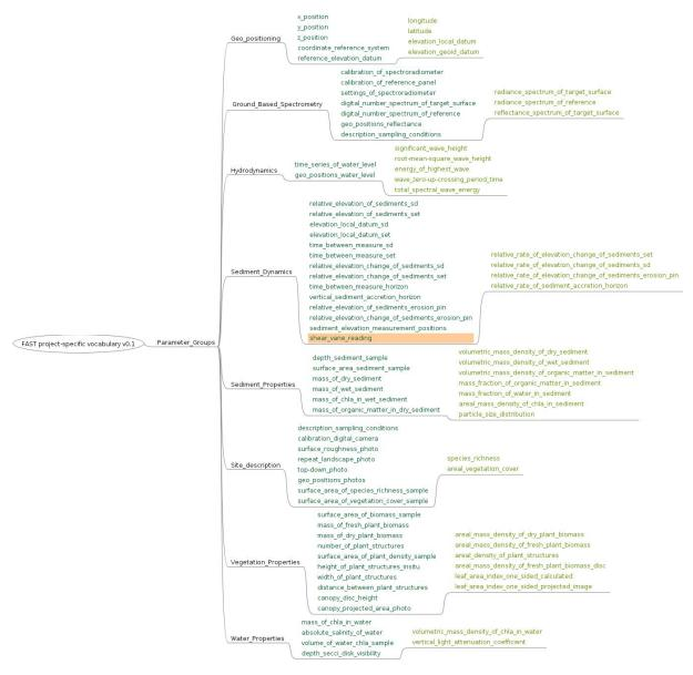
Figure 12: Schematic of grouping and naming conventions adopted for the parameters measured in the field. Black indicates parameter group, dark green indicates L0 parameter names, light green indicates L1 parameter names.
