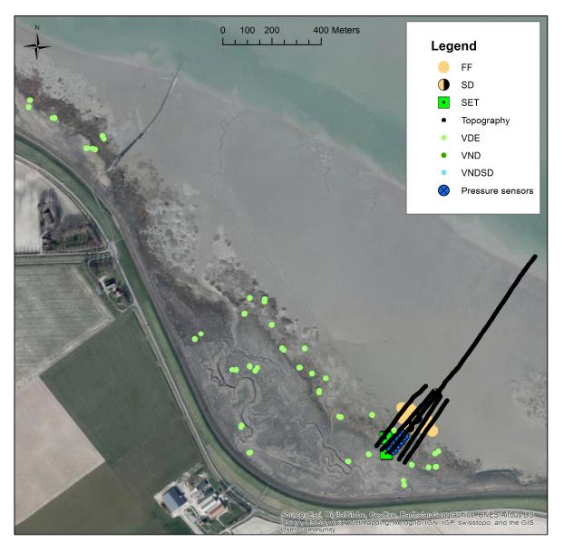
Figure 10: Locations of topographic surveys, monitoring equipment and sampling quadrats deployed at NL Y1 site
