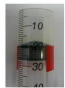
Figure 16: Sediment sampling with the big syringe, sides of the plunger should be level with top of the red tape to sample the right volume, as shown here.
