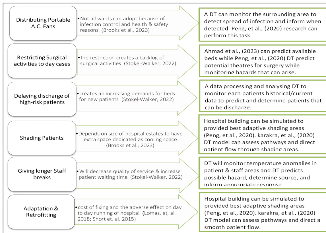
Figure 5 Using digital twin to answer some challenges experienced by hospitals during heatwave.
