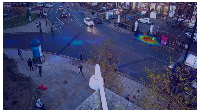
Fig. 18. Heatmap representation of areas in which vehicles and pedestrians were too close to each other. Source: 10,000 live video frames from Leeds dataset.
