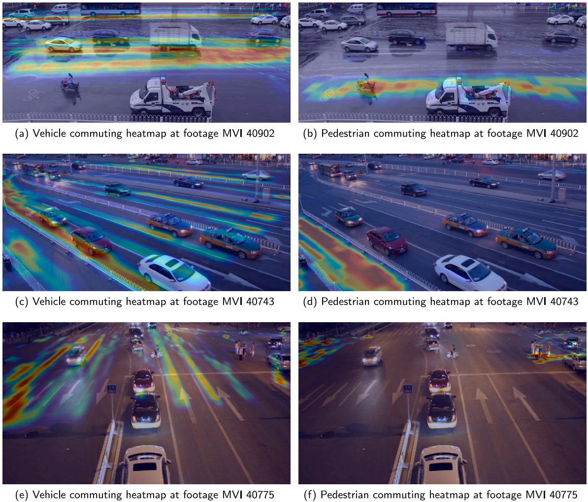
Fig. 15. The analysis results for UA-DETRAC (Wen et al., 2020) datasets video footage. The Left and Right columns are the heatmap representation of vehicles' and pedestrians' movements, respectively.
