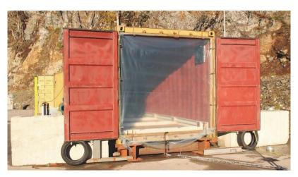
Figure 7: Container doors in fully open position, and opening covered by a polyethylene sheet.
