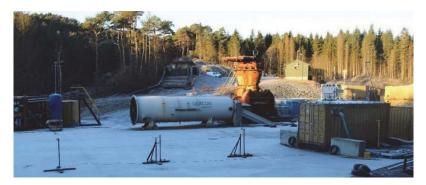
Figure 2: Test site with a 20-foot container and supports for the three external pressure sensors.
