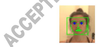
Figure 2. Output of the face detector algorithm drawn from the left robot eye camera; blue circles represent the detected position of the eyes.
