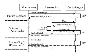
Fig. 2: Sequence Diagram of Runtime Controlling Model
