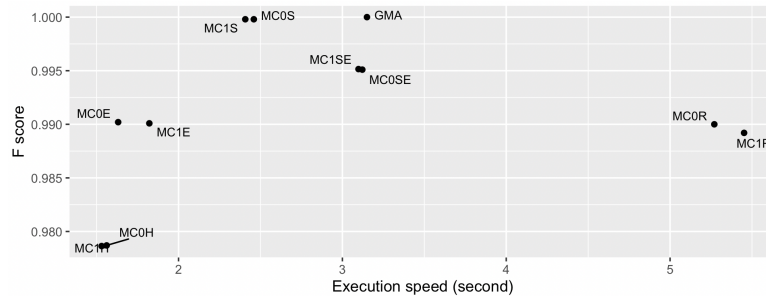
Figure 3: Pareto comparison of optimal instantiations of the matching algorithms. Optimal GMA parameters: MIS = 1 , MIP = 1 , PIS = 0.8 , MSD = 0.25 , MCCF = 0.8 ; MCOSE: Multi-Criteria ( d_b = 0 ) with Surface and Eucliden criteria.
