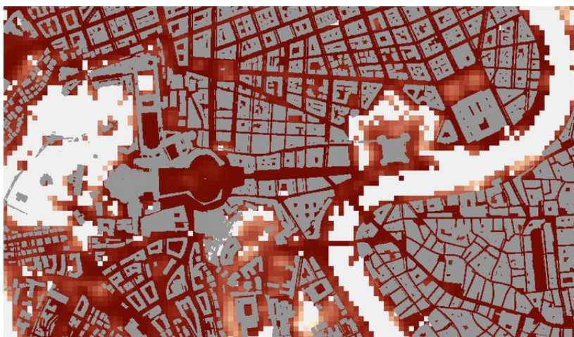
Figure 14: Screenshot comparing the HRL imperviousness product (red), capturing all sealed areas, with the Building Layer (grey), offering more detailed information on the built-up structures. Source: CLMS.
